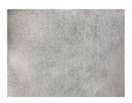
DeWitt Supreme (or N-Sulate) is a 1.5oz spunbond polypropylene fabric used primarily for plant protection.
